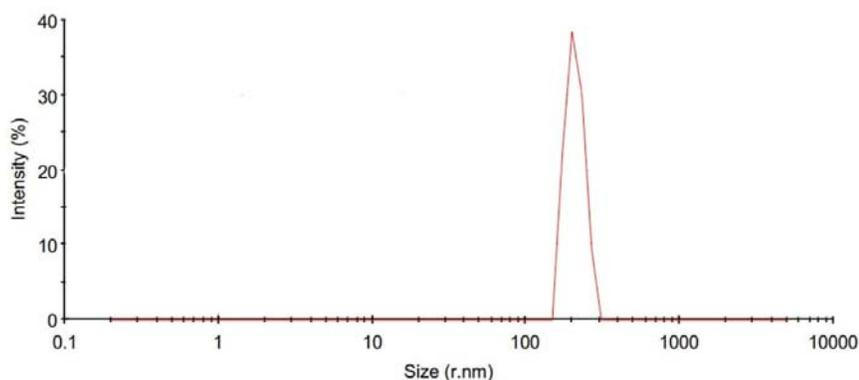
**Fig. 1.** Size distribution of the chitosan-JQ1 nanoparticles was measured by the Malvern Zetasizer instrument. The particle size (nm) is represented by the horizontal coordinate and the intensity is represented by the vertical coordinate (%). All particle sizes are concentrated in the range of one peak.
