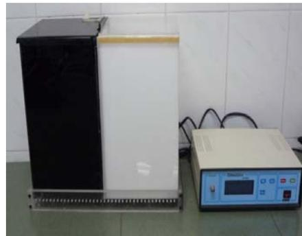
**Fig. 3.** Passive avoidance apparatus.
