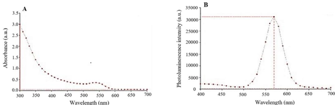
**Fig. 1.** (A) optical absorbance and (B) photoluminescence spectra of CdTe QDs. These results were obtained under excitation with ultraviolet light (360 nm). The absorption edge occurs at ~ 540 nm (A), and the maximum emission peak occurs at ~ 570 nm (B). CdTe, Cadmium telluride; QD, quantum dot.
