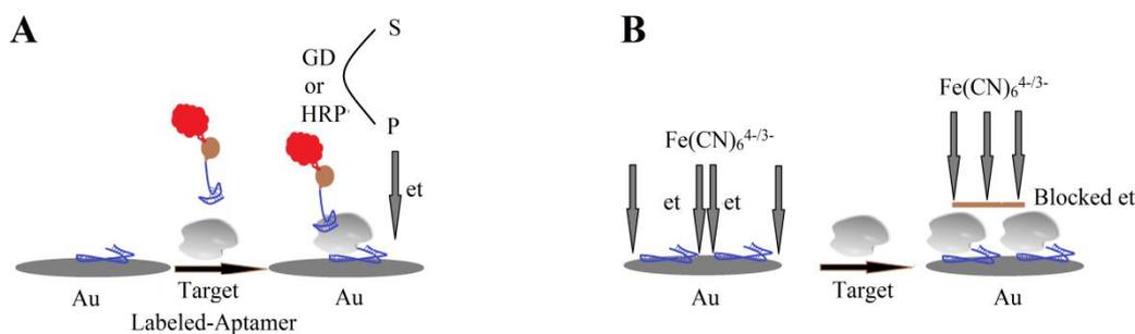
**Fig. 3.** Schematic picture of electrochemical biosensing. The interaction between aptamers and targets impact electron transfer to the gold nanoparticle coated electrode, making signals proportional to the detected targets. (A) Conjugated aptamer-based approach in electrochemical biosensing and (B) free aptamer-based approach in electrochemical biosensing. HRP, Horseradish peroxidase; GD, glucose dehydrogenase; et, electron transfer; Au, gold;  $\text{Fe}(\text{CN})_6^{4/3-}$ , Ferrocyanide.
