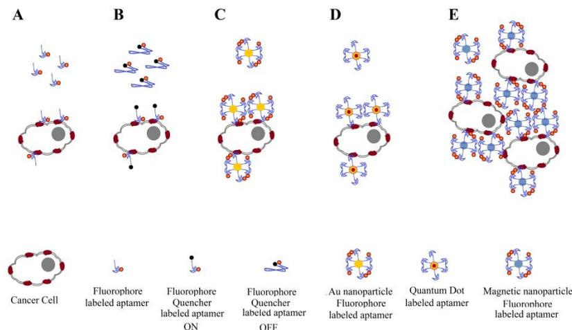
**Fig. 4.** Schematic picture of fluorescence biosensing. Various types of fluorescence biosensors are depicted as described in the picture. (A) Simple fluorophore-labeled aptasensors; (B) fluorophore/quencher-based aptasensors; (C) gold nanoparticle/fluorophore-labeled aptasensors; (D) quantum dot aptasensors; and (E) magnetic nanoparticle/fluorophore-labeled aptasensors.
